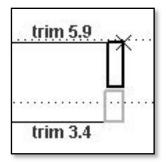
It shows the space occupied by the MSX subs. The size of the rectangle expands depending on how many MSX may possibly be above the MLA Mini, one for four Mini, two for eight Mini and so on. The rigging tab allows accurate calculations when this mode is selected as we will see.
