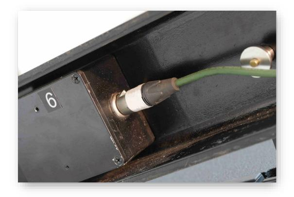
Connect one of the 800mm AES XLR cables and an 800mm U-Net cable (usually loomed together) from the audio out and U-Net port 2 on the top MLA cabinet down to the Audio input and U-Net port 1 on the second cabinet;-
