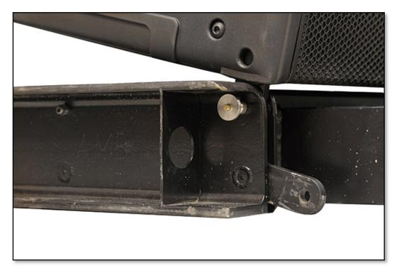
Now connect the MLA ground stack bars to the appropriate holes in the grid just under the rear of the MLA. Raise the rear of the cabinet and pin the bar into the hole in the MLA as required to obtain the necessary angle;-
