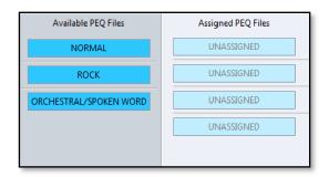
It is important to do this not only to add some tonal EQ to the system but the PEQ synchronisation also performs a reset function on certain parameters in the array. It matches the input setting for every cabinet in the array to the first enclosure and resets the array delay to the default setting. Here we have applied the Rock PEQ to all arrays;-
