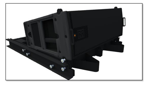
You are now ready to set the angle at the rear using one of the two ground stack bars. There is a long and a short bar the use of which is determined by your Display 2.1 design. If the bottom cabinet has an upward tilt the short bar is used, if it has a downward tilt the long bar is used.
