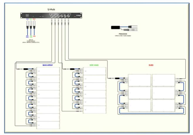
Audio input can be direct from a console or from a DX4.0 processor used as a matrix. Three audio feeds – each either balanced analogue or AES EBU digital- are connected to the three audio inputs on the rear of the U-Hub.
