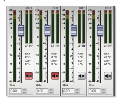
There is also a temperature read out showing the temperature of both the DSP and amplifier module;-
