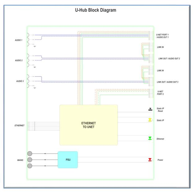
U-Net is run as a redundant loop, all U-Net enabled products have two ports. Port 1 on the U-Hub would be connected to port 1 on the first device, port 2 on this device would link out to the next device and so on with a final link back to port 2 on the U-Hub to complete the loop. This allows the system to continue working seamlessly in the event of a cable being damaged or inadvertently disconnected. Data will simply flow in the opposite direction to allow continuous communication.
