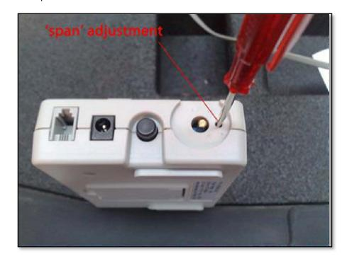
Carefully adjust the pot until the display matches the reference. Next lower the grid to around -30° and -20° checking each time that the reference and reader displays match. It may be necessary to re-adjust the zero measurement following calibrating the span, in which case check the span calibration again.
