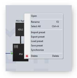
'Open' functions in exactly the same way as double clicking on the cabinet icon and opens the PSX overview screen to allow detailed control and monitoring
