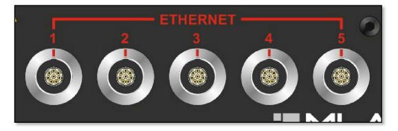
These are fed from the Ethernet switch which also connects the Merlin and Wi-Fi components so all are available on a single Ethernet network. From this connection point you can connect to the PC and to all slave racks being used, most frequently a single Slave on the opposite side of the stage. Any network cable can be used for Ethernet connections excluding the 120m PWA00041; the maximum cable length for Ethernet is approximately 100m.
