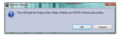
If you click on OK, all gain and delays will be restored to zero, any inverted outputs will be re-inverted and any muted outputs will be un-muted.
