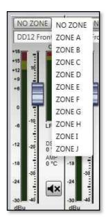
Click on the desired zone and it will be displayed on the zone button. The zones are colour coded to make it instantly obvious which cabinets are on the same zones. Colours are as follows;-
