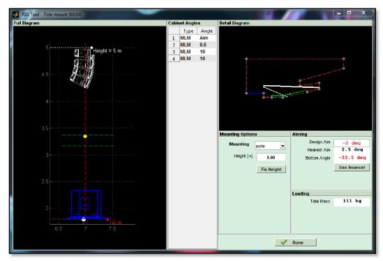
We can see that the array is far too high to fit on the standard pole so the first job is to correct the height to something that is usable in the real world. This is provide for pole mount deployment by the 'Fix Height' button;-
