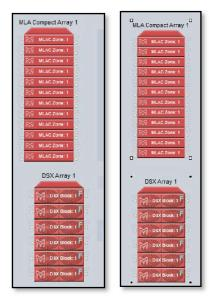
Again the arrays are not very well aligned but a simple click of the vertical alignment button and they are perfectly in line.
