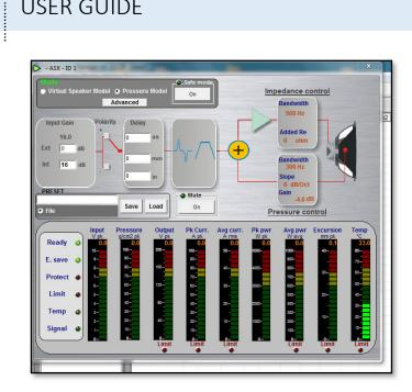
Click on the 'Load' button and navigate to the file "MLX\_A02.pow" in the un-zipped upgrade folder;-
