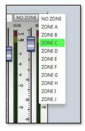
Click on the desired zone and it will be displayed on the zone button. The zones are colour coded to make it instantly obvious which cabinets are on the same zones. Colours are as follows;-
