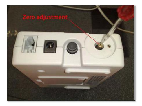
This is supplied by the manufacturer with an adjustment knob but this may have been removed by Martin Audio so that once calibrated the controls can be covered with a label to prevent accidentally changing the calibration. If the knob is still present carefully remove it as you will need it out of the way for the span calibration. Using a small screwdriver, adjust the control until the read-out exactly matches the reference level.
