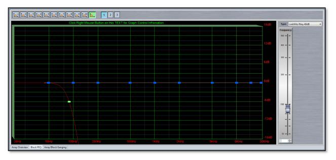
There are also ten PEQ filters at your disposal, each with exactly the same functionality and control. The low pass filter in common with the high-pass in the MLA, MLD and Compact, can be either Bessel, Butterworth or Linkwitz Riley with slopes from 6dB per octave up to 48dB per octave. The frequency can range from 50Hz up to 500Hz;-
