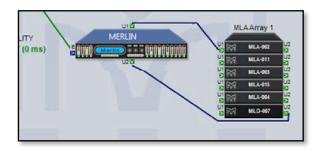
The U-Net ports on the Merlin are on the top and bottom of the Merlin icon, in most cases this allows Vu-Net to draw the system connections neatly as in the above example but they may be instances where the position of the arrays and complexity of the system means that the network connections cross and the system diagram looks untidy;-
