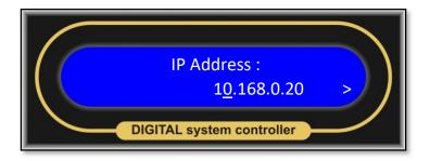
You will notice that the least significant digit of the first range is underlined. Use any of the three control knobs, 'Freq', 'Q' or 'Gain' to adjust the number, then using the 'Right' button shift to the next range and adjust. Continue until the IP is in the same range as your PC but not exactly the same for example 10.10.10.33. Press 'Enter' to return to the Network Settings submenu. Press 'Enter' again to check that the settings are correct;-
