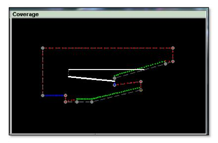
When you start the optimisation process which window switches to an index plot showing in real time the acoustic performance as different inter cabinet angles are tried;-
