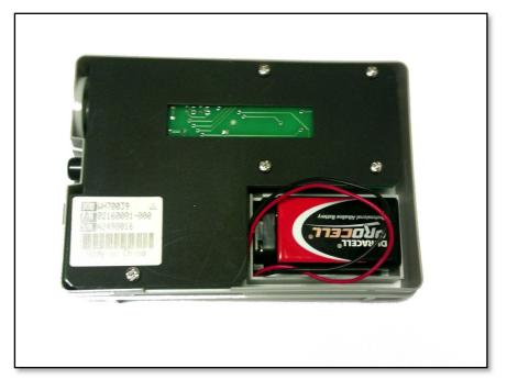
Ease the battery out, pull the clip off the terminals, clip the new battery onto the battery lead and replace it in the upper half of the case. The bottom is fitted back on and clips into place. Turn the reader on to check the new battery has been fitted correctly and is working ok.
