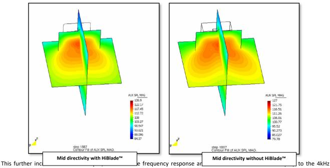
crossover point. This is high for a midrange horn and is key to enabling the use of 1"compression drivers for reproduction of high frequencies. MLA's 6.5"cone/1"compression driver combination replaces the more traditionally used large format compression driver and has less distortion, as well as having a much more extended HF response.
