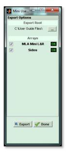
The First step is to create a file into which the D2P optimisations will be loaded. The Export Root defaults to your PC C: drive but it is good practice to save your files to a dedicated folder which can be used to store all files created for a particular project. Click on the small box on the right of the Export Root section, navigate to a convenient file location, and if necessary create a new folder first to drop the file into. The Export Root will show the file location;-
