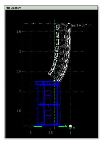
As with ground stacked MLA and MLA Compact ground stacked systems, if the array is not already locked to the ground using the option in the Slice tab, you can select it here;-
