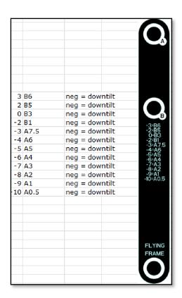
In the example we have shown we need to achieve an angle of  $-2^{\circ}$ , we would therefore use hole 'B' on the ground stack bar connected to the  $1^{\circ}$  hole on the bottom cabinet.
