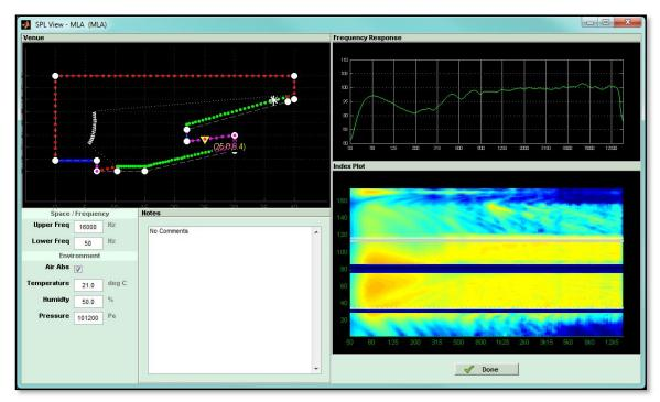
As you can see, the response right to the back of the balcony is incredibly flat from around 500Hz and above. Below the frequencies at which the optimisation is effective there is the expected low frequency roll-off but the mid-top response is incredibly consistent
