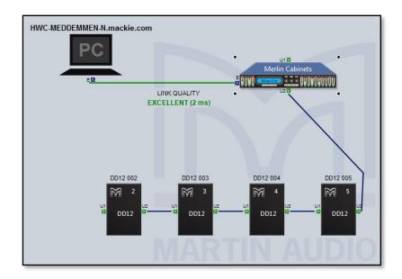
Each DD12 icon in the overview screen features a Martin Audio logo. Double-clicking on this will illuminate the LED on the cabinet front grille to assist in identifying each DD12 which is very useful when multiple units are deployed.
