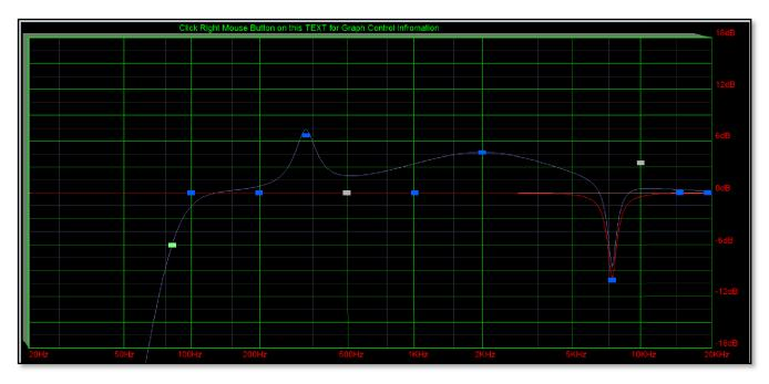
The horizontal axis is frequency in Hertz from 20Hz to 20KHz, the vertical axis is gain from -18dB up to +18dB. Colour coding is also used on the graph to represent the various modes.
