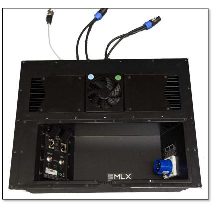
The module is held in place behind the ventilation panel and connector lid, removal is a simple case of unscrewing the fixing screws and disconnecting the two Neutrik NL4's which connect the drivers and LED's to the module, the Neutrik p-pin XLR which connects the iPal pressure sensor and the Cat 5 cable that links to the iPal data port. Field replacement therefore is very quick and easy in the unlikely event of a module failure.
