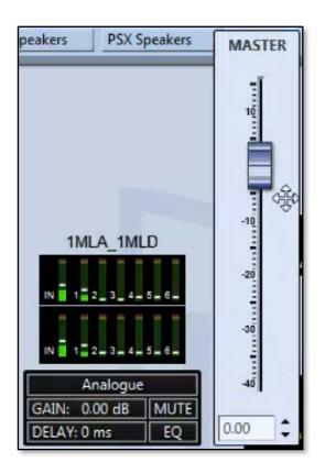
Using the up/down arrows to adjust the gain up or down in 0.1dB increments;-
