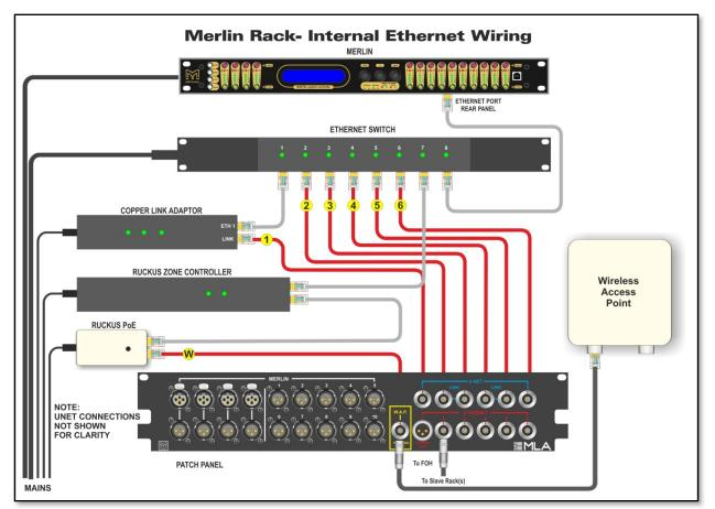
This shows the WAP which is supplied as part of the FoH rack. There are similarities with the Mk1 system with the Ruckus Zone Director replacing the PicoStation DHCP Server. The feed to the WAP is via the WAP PoE and goes to a dedicated antenna connector on the patch panel. This also has 48V present so should not be connected to other Ethernet devices.
