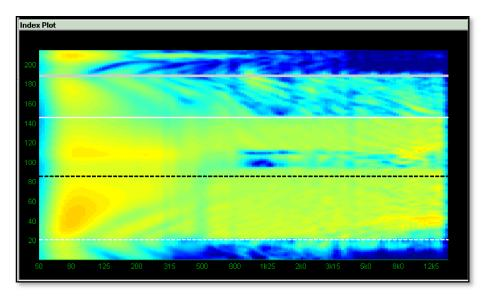
And to demonstrate how close the system can get to the perfect coverage, here is the same venue with an array consisting of 16 MLA plus 1 MLD optimised to obtain a front to back differential of 0dB- exactly the same spl everywhere. The audience target has been given maximum priority ignoring non-audience and hard avoid areas;-
