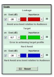
The three goals are Leakage, Target and Hard Avoid. The relative balance for each of these is controlled by the horizontal faders with the numeric percentage value of each showing to the right. The default starting position is each with equal importance so a level of 33% for all three (yes that equals 99% not 100, get over it...).
