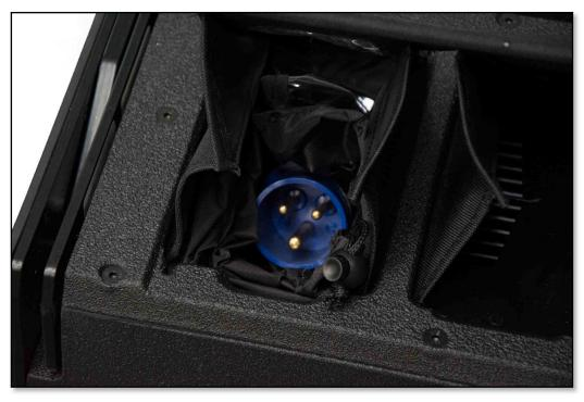
The MLA Compact has a universal PSU suitable for direct connection to virtually any mains voltage anywhere in the world. If you are not using the Martin Audio MLA distribution system a matching Ceeform 16A female outlet connector must be used. For outdoor use this should be rated at IP67, this is to ensure safe operating when any connectors are disconnected in damp conditions.
