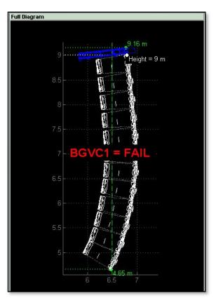
In this case it is necessary to chance the height and possibly coverage area of the array until a "legal" array shape is produced or in the case above, reduce the number of cabinets or switch to a two point hang.
