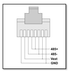
This is easily achieved by using a standard CAT5 patch cable, cutting off one end, stripping back the connectors and wiring into the terminal block on the EasySync adaptor is used. This is very much quicker and easier than having to make up a custom RJ45 to 9-pin D-type cable. The cable connections for RS485on the EasySync are as follows;-
