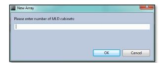
Enter the number of MLD required in the array. In the majority of systems this will be one or two. They will automatically be added to the bottom of the array.
