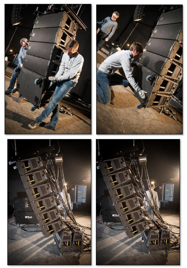
When you have connected the final Compact, connect the last Ceeform connectors to all remaining cabinets and the last link then the final U-Net cable that goes back up to the array loom checking for U-Net connectivity both on Port 2 of the final cabinet and on the Merlin.
