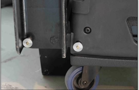
Make absolutely certain that the pin is properly engaged with the centre button out in the locked position. Give the pin a firm pull to make sure it cannot come out. All pins should be checked at every stage of the rigging process. Any with the centre button depressed;-
