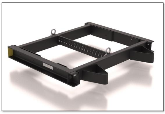
The MLA flying Grid is the principal system for deployment of MLA systems. When used with a two point suspension system it can be used to fly up to 24 MLA or 15 MLX or a maximum of 6 MLX with 12 MLA flown below in a combination array (note that this configuration requires two grids). The grid features a central spine which allows single point rigging of up to 10 MLA.
