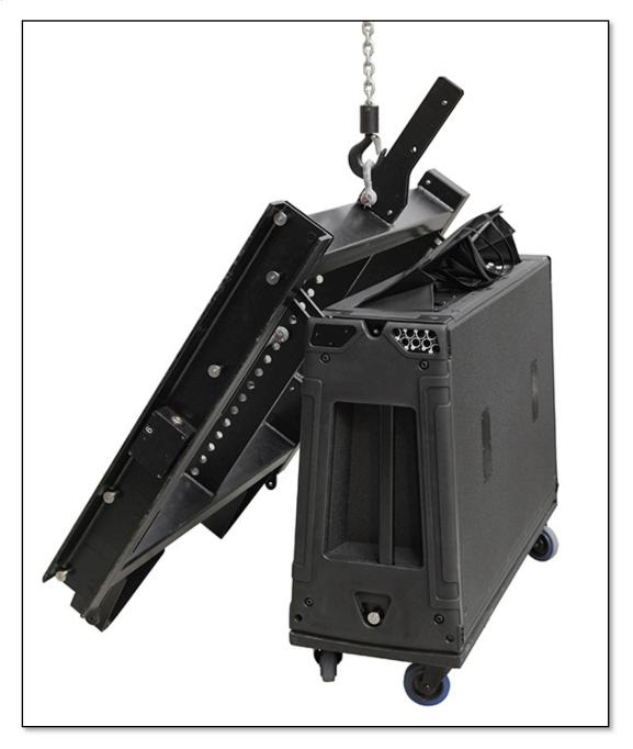
Connect the rear bracket to the holes at the back of the flying grid. As the cabinet is at the back of the grid it is impossible to line up the front rigging positions with the cabinet and grid vertical, it is also difficult to swing up the cabinet to the grid as the grid has little stability with no cabinets attached so it will move around making it awkward to fir the pins. The easiest option is to fly
