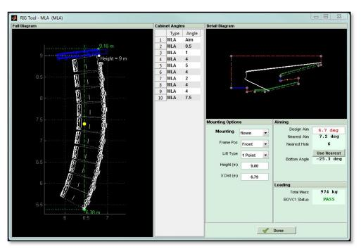
There are a number of important sections to the screen. First is the array diagram showing a scale picture of the flown array accurately displaying the physical deployment of the array;-
