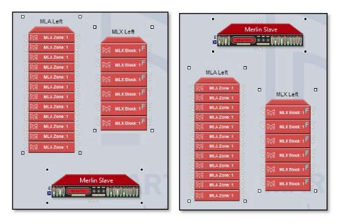
The third button applies only to the Merlin. When a system is discovered on line all U-Net connections are shown from the Merlin to all arrays;-
