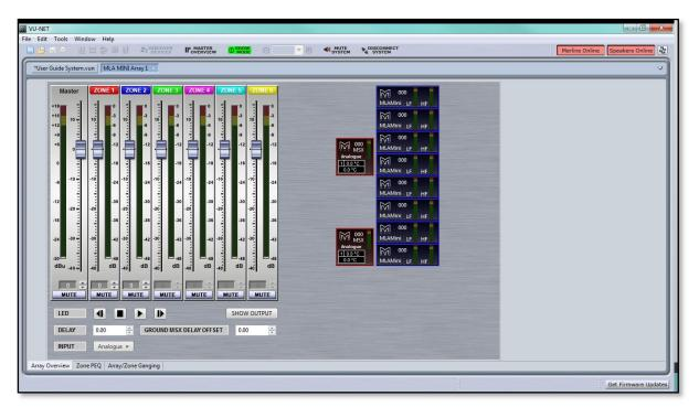
As you can see, the main array window is almost identical to the other MLA System components; there are the usual six zones available each with a gain fader and mute switch. Unlike other cabinets the faders are present at all times regardless of whether anything is assigned to them. The difference is that un-assigned zones have the gain read-out above the mute button greyed out. If you attempt to adjust gain or mute an un-assigned zone you will see the following window;-
