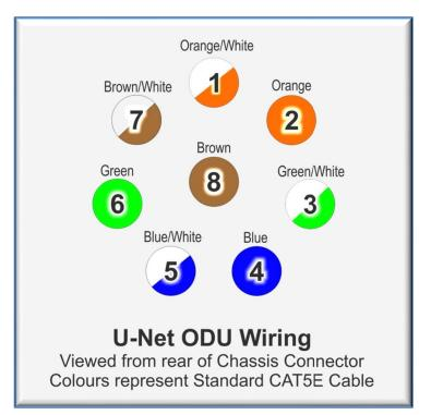
The two pairs of linked ODU connectors are wired as shown in the block diagram. Pins 1, 2, 3 & 6 are linked together, pins 4 and 5 on the link out connectors have the audio signal from the corresponding audio input.
