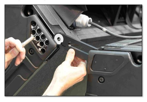
Check which hole needs to be connected from the optimisation that you did with Display 2.1 and connect the rear brackets with the flying pins;-
