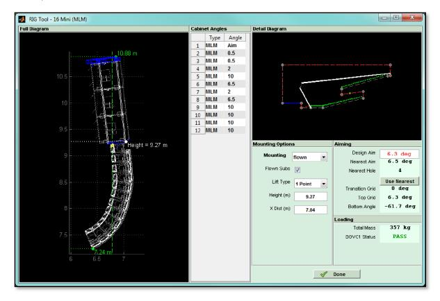
As with MLA and MLA Compact systems you can select 1 or 2 point hangs, the difference is that even with the maximum flown MLA Mini, either 16 alone or 12 with 3 MSX, they will still be within BGVC1 limits from a single point. 2 point does of course give you the flexibility of trimming the array angle by fine adjustment of one or other hoists.
