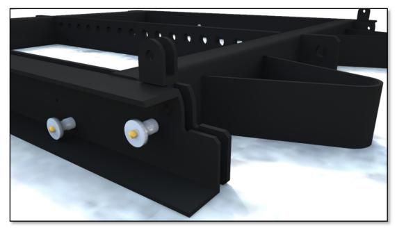
Now place the first cabinet flat on top of the grid being careful that the exposed bracket doesn't damage the bottom of the cabinet, always lift it into position rather than dragging it. Secure it into the bracket at the front of the grid with a flying pin;-
