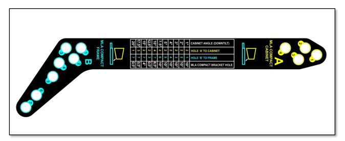
There are a number of options that are used to obtain the correct angle; the angle is shown in the first column, having selected your angle you then look across to the next three column which show you which of the cabinet connection holes "A"(yellow) from 1 to 4 to use and which of the Frame connection holes "B"(Blue) from 1 to 7 and finally which bracket hole in the bottom cabinet to use.
