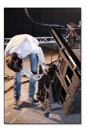
Raise the array just enough to get the Compact clear of the floor and swing the two cabinets up pinning the 3<sup>rd</sup> cabinet to the 2<sup>nd</sup> at the front on both sides;-
