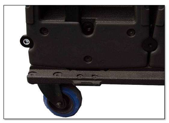
The cabinets are joined using machined quick-release pins. There are an identical design to the MLA pins but a smaller size. These have spring loaded ball bearings at the end of the pin which protrude beyond the outer diameter of the pin thus locking them in place. To release them, the central button is depressed whilst pulling the pin clear using the wide flange. This is best done with
