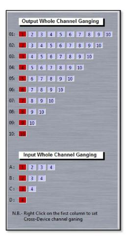
In the default state there is no ganging, each input and output is essentially ganged to itself as indicated by the red squares in the left hand column. To gang output channel 1 to channels 2, 3, 4, 9 & 10 for example, click on the relevant squares in the horizontal line by output channel one;-
