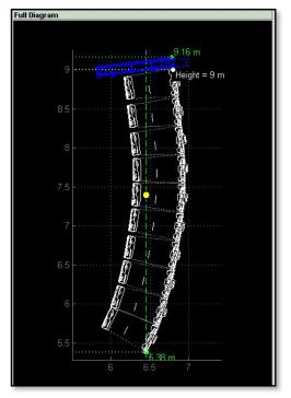
This is useful so you can quickly see if there are any mechanical issues with the array that might make flying in a particular venue difficult; perhaps the rear of the array is hanging back further than you initially thought and might impede something else that
