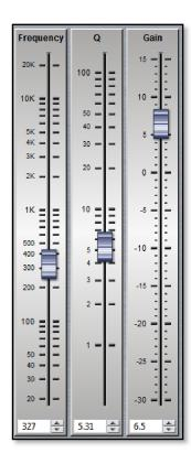
Parameters can be changed on the properties panel in three ways. The faders can be drag and dropped to a new value, the value can be scrolled up or down using the up/down buttons to the right of the value windows, and finally values can be directly typed into the value windows. The response graph will adjust according to the new values and vice versa, adjustments in the graph window will be reflected in the fader positions and values in the properties panel.
