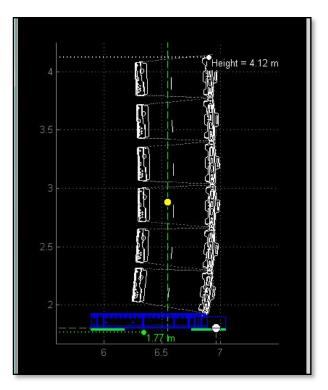
'On Ground' refers to the lowest point on the venue slice available for the horizontal (front to back) position for the array. If for example the array is placed on a stage, selecting 'On Ground' will result in a Lower trim equal to the stage.
