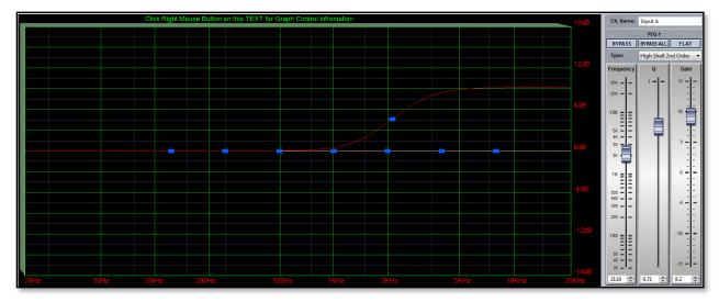
Low Shelf 2<sup>nd</sup> Order is a low shelving filter also with +/-15dB of gain and Q factor from 0.25 to 1.0;-
