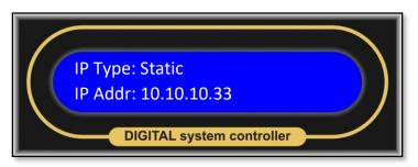
Three presses of the 'Back' button will return you to the main menu. Power cycle the Merlin and return to the Network Settings submenu to double check that the settings are correct.
