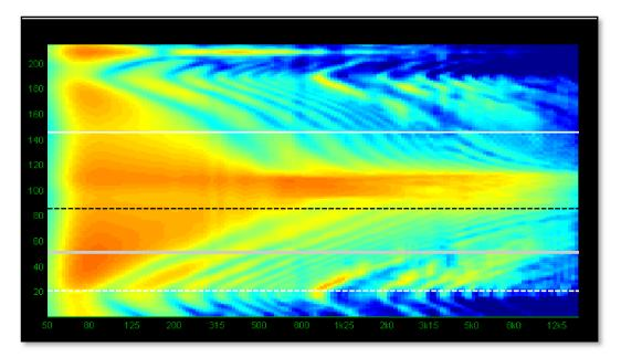
This is the Index plot of a completely un-optimised system. The horizontal axis as mentioned is frequency. As we cannot optimise very low frequencies the graph starts at 50Hz going all the way up to 20KHz. The vertical axis is now the 2D slice of the venue
