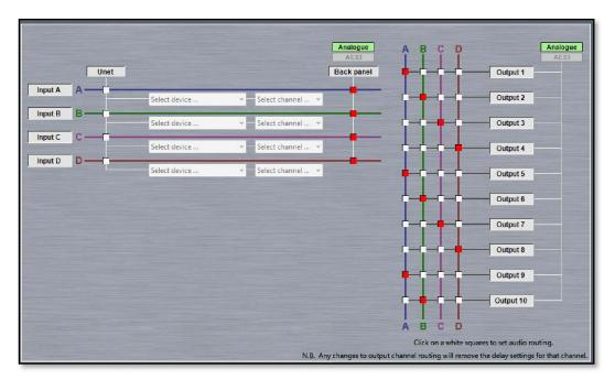
As with All other MLA devices, the Merlin has the facility to accept a digital input over the U-Net network ready for when this feature is implemented. This is achieved by selecting the Unet option which can be done individually for each channel;-
