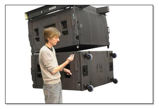
An easier option is to fly the array until the second cabinet is just off the ground, swing it forward and immediately land the array with the second cabinet horizontal so the first cabinet sits on top of the second;-
