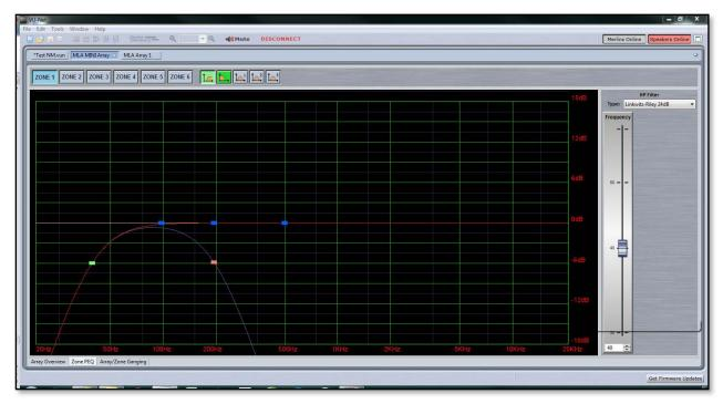
It is a slightly simplified version of the PEQ Tab that is available in all other array components. The six available zones can be selected by using the Zone buttons at the top of the window;-
