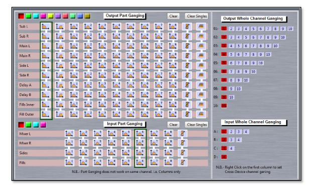
There are three types of ganging available, whole input and output ganging, Part input and output ganging and cross device ganging which enables you to mirror the parameters programmed into one Merlin across one or more other Merlins on the same U-Net network. Ganging duplicates the settings on ganged channels or parameters. There is no "Master" and "Slave" system parameters can be adjusted on any channel, parameter or device and any ganged channel will match the setting.
