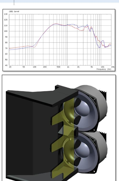
Another feature of MLA's midrange horn is the HiBlade<sup>™</sup> device, which modifies the wave-propagation in the horn throat.
