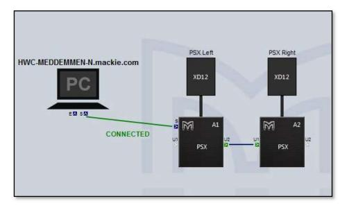
Each PSX icon in the overview screen features a Martin Audio logo. Double-clicking on this will illuminate the LED on the cabinet front grille to assist in identifying each PSX which is very useful when multiple units are deployed.
