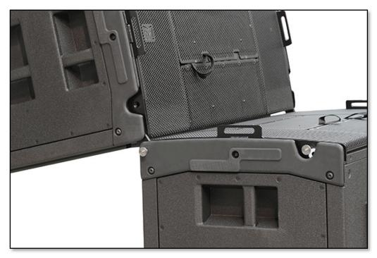
There are now two options for attaching the front rigging. It can be flown off the ground and the second MLX swung up and connected at the front in exactly the same way as MLA however this requires strong crew as the MLX weighs 160Kg.
