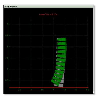
When it has completed its first pass it will start again on its polish cycle if you have checked this option. The array will change colour to yellow. When the optimisation is finished you will see the array diagram with the array now stationary. The yellow polished version will be superimposed above the green un-polished version. The accurate lower trim height is also displayed;-
