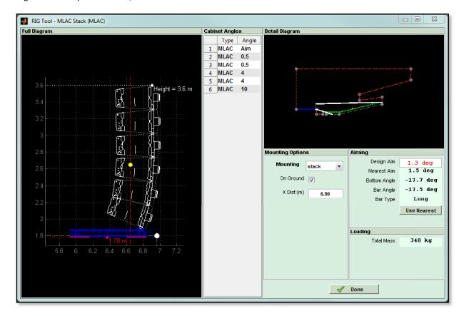
The principal difference is how the ground stack information is displayed. MLA Compact has two versions of ground stack bar, a long bar for arrays requiring a down-tilt as shown in the example above, and a short bar for arrays that require an up-tilt. As the example above shows, the Aiming panel shows which type of bar;-
