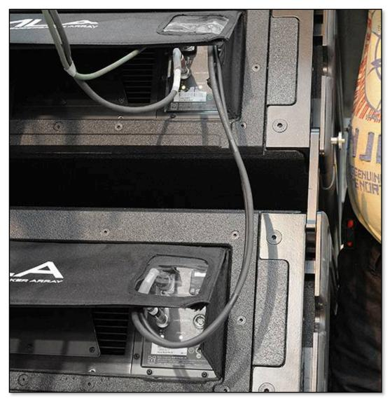
At this point the U-Net ports will not light on either cabinet as the second cabinet is not yet powered.
