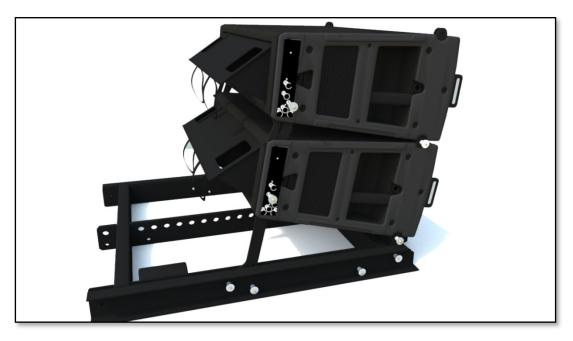
Continue adding cabinets, always connecting the front brackets first and then setting the angle and pinning at the rear;-
