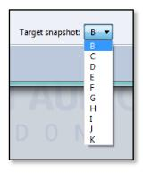
There are ten available labelled from B to K. A is the default factory preset with basic box EQ which may be used whilst checking a system or in an emergency, all other are available for your optimisations and once uploaded can be selected in a few seconds. Select the desired location using the drop down button.
