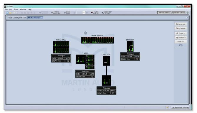
The MLA array shows the input bargraph plus all Cell output bargraphs for all cabinets in the array, all other arrays and speakers show input and output levels and all Merlins display input and output meters. All bargraphs are updated in real time which makes monitoring an entire system very easy from a single page.
