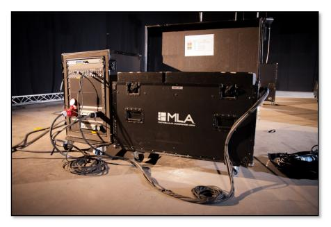
Connect the Tourmate mains cable to the mains distro, U-Net cables to U-Net ports 1 & 2 on the patch panel and the inclinometer cable to the reader which can be placed on top of the rack. If you are using the Merlin in the rack for audio distribution you can connect the array audio feed to the relevant audio output on the patch panel;-
