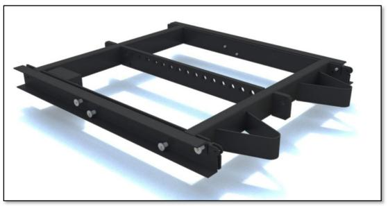
The MLA Compact flying Grid is supplied in pairs with all MLA Compact systems. It enables flying of up to 24 MLA Compact when using a two point lift, or 12 enclosures from a single point. Ground stack systems of up to 6 Compact can also be employed using the same grid with the addition of ground stack bars which as supplied as part of the system.
