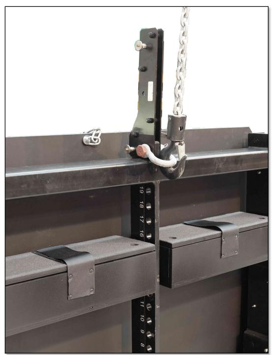
Raise the hoist until the grid is just clear of the flightcase. Roll the flightcase out of the way and lower the grid until it is just resting on the two 'V' shaped bumpers on the front. Do not allow the chain of the hoist to become too slack, not only will it get in the way but keeping it taught will provide additional support for the grid to prevent it falling over when it is upright;-
