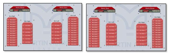
The left hand shot shows a system drawn with the left and right arrays placed on the wrong sides, the right shot has been corrected with the reverse order horizontally button.
