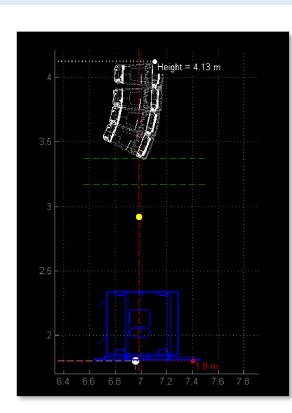
Note that the array height displayed is the height from the ground NOT above the MSX. You can see that the MSX is at 1.8m, perhaps on a stage so the top trim of the array is at 4.13 - 1.8 = 2.33m above the surface on which the MSX is placed.
