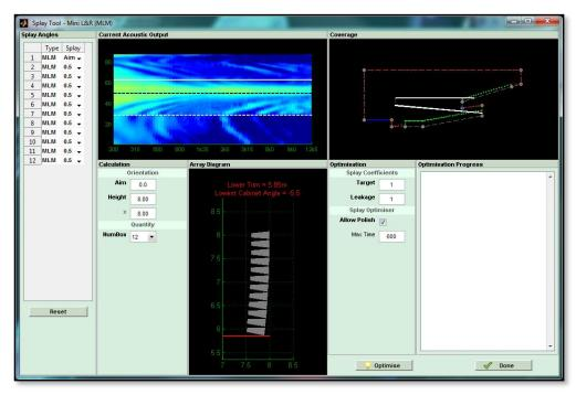
There are a number of sections to the window, these are;- Splay angles, Current Acoustic Output, Optimised Acoustic Output, Calculation, Array Diagram, Optimisation and Optimisation Progress.
