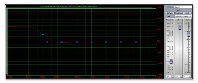
There are no dedicated high and low pass filters on the inputs but High pass and lowpass with variable Q are options for filter types;-
