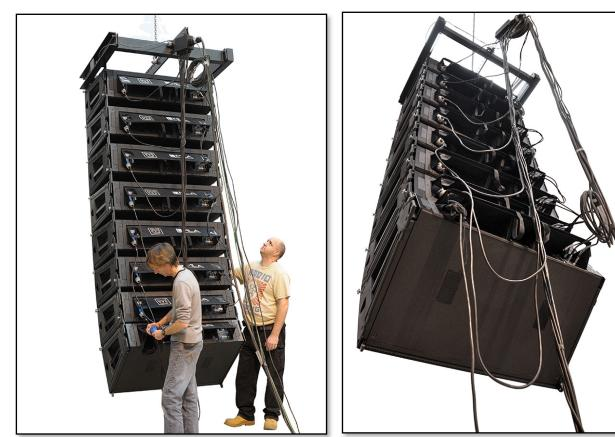
When you arrive at the final cabinet the only difference is that the trailing second U-Net cable is connected to the final U-Net 2 port on the last cabinet and the U-Net LED should be checked for good network connectivity between the final cabinet and U-Net port 2 on the Merlin back in the rack.
