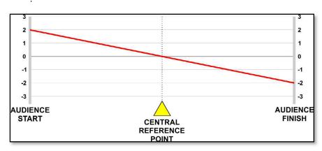
This shows a system that has been set up with the reference point in the centre of the audience region and a start and finish delta of + and - 2dB respectively. Because the reference point is central, the SPL drops evenly from start to finish, down 4dB from the loudest point at the start of the coverage.
