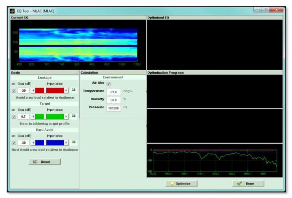
The Current EQ section shows the system response that we saw when we had finished the splay optimisation. The blank windows to the right will show the Optimised response as the optimisation is taking place.
