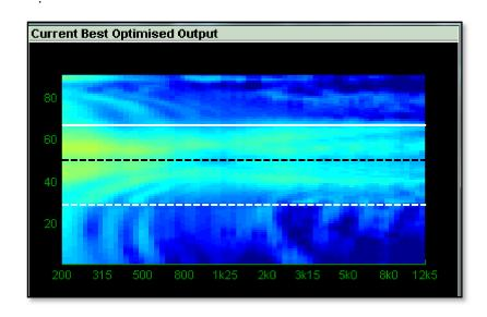
This gives you an instant comparison to the Current Acoustic Output; essentially a "before" and "after" to see how manually articulating the array has improved the coverage.
