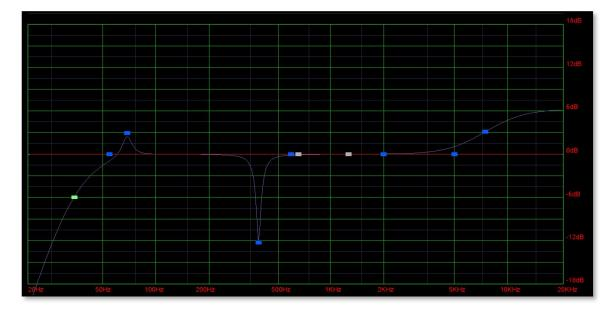
The horizontal axis is frequency in Hertz from 20Hz to 20KHz, the vertical axis is gain from -18dB up to +18dB. Colour coding is also used on the graph to represent the various modes.
