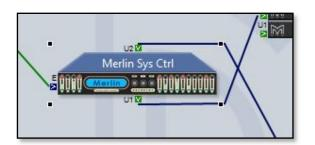
If this is the case, select the Merlin and click on the 'Reverse U-Net ports' button and the port position is reversed in the system diagram hopefully making the network connections look neater;-
