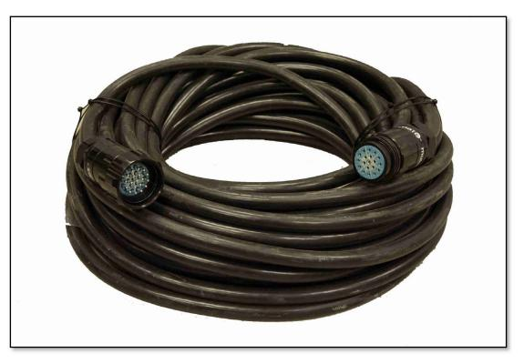
**ASF12002** is a 30m 18-core multiway mains cable terminated with Tourmate 19-pin connectors, one male, one female. Tourmate is based on the popular Socapex pattern but is rated at IP67 when mated so if suitable for use outdoors in all weather. The cable has 18 cores each 2.5mm<sup>2</sup> and has a tough, flexible outer sheath. Other lengths are available to special order. The Tourmate is used to connect a Master or Slave rack to an array.
